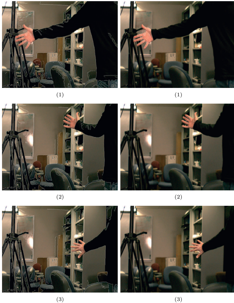
Fig. 6.6. Second example of hand edges extraction in cluttered background: edge detection (left column) and the extracted hand edges (right column).
