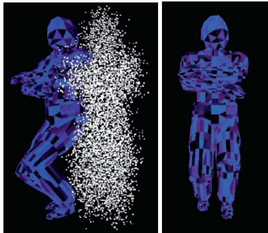
Fig. 14.10. Starting pose on the left with the disturbed point cloud of the target pose (noise deviation 0.05 m) and target pose on the right.
