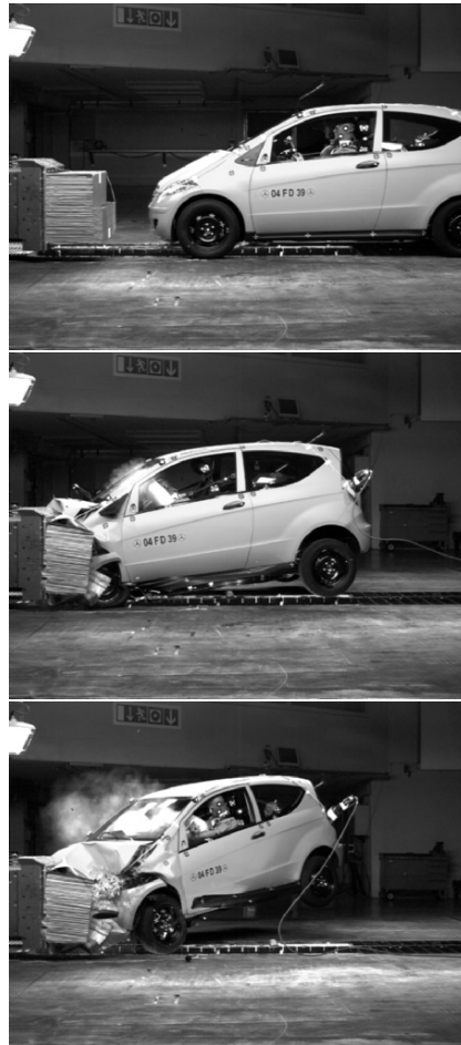
Fig. 19.6. First and last frame of an A-class offset crash sequence. The middle image shows the moment of deepest air bag penetration.
