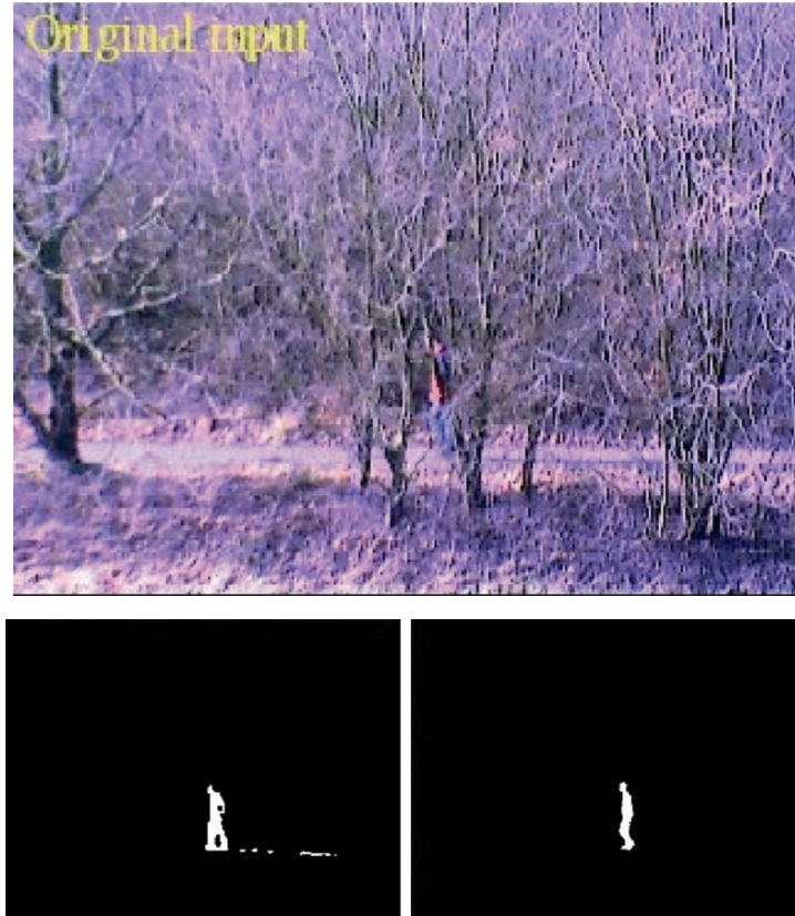
Fig. 3.3. This image shows an example of normal occlusion and shadow. The top image shows the original input image. The bottom left image shows the normal output from the background subtraction function while the bottom right one shows the detected silhouette, parameterized according to the detected parameters.
