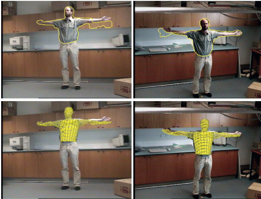
Fig. 11.3. Result with a two-step approach, i.e., extraction of the contours from the images followed by contour-based pose estimation. The same initialization as in Figure 11.2 was used. Top row: Estimated contour. Bottom row: Estimated pose. As pose and contour are not coupled, the contour extraction cannot benefit from the two camera views. Moreover, as the contour is not bound to the surface model, it can run away.
