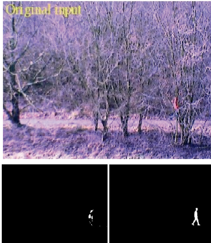
Fig. 3.2. This image shows an example of normal occlusion and shadow. The top image shows the original input image. The bottom left image shows the normal output from the background subtraction function while the bottom right one shows the detected silhouette, parameterized according to the detected parameters.
