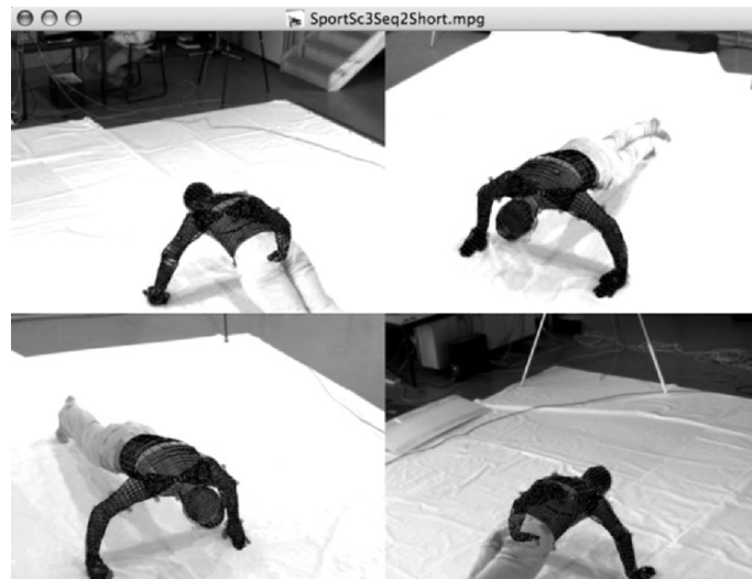
Fig. 1.17. Human poses are tracked using a generic 3D model of the upper human body; the figure shows the backprojection of the recorded 3D motion into the original 4-camera image sequence, also demonstrating model movements of occluded body parts [39].
