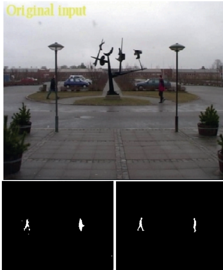
Fig. 3.4. This image shows an example of heavy occlusion. The left image shows the original input image, the middle one the normal output from the background subtraction function, the right image shows the detected silhouette superimposed.
