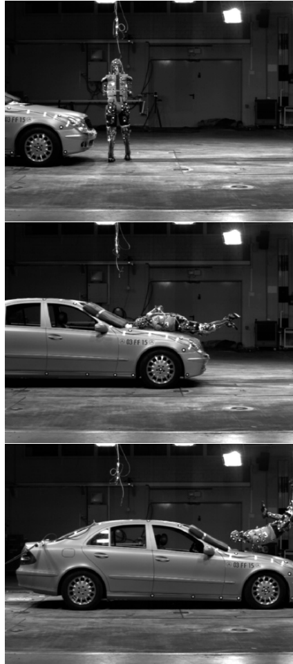
Fig. 19.11. Frame 0, 100, and 200 frame of a pedestrian crash sequence. The sequence was recorded at 500 Hz and the vehicle speed was 36 km/h.
