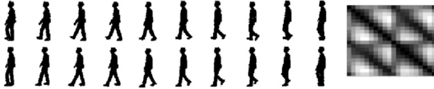
Fig. 2.1. Twenty sample frames from a walking cycle from a side view. Each row represents half a cycle. Notice the similarity between the two half cycles. The right part shows the similarity matrix: each row and column corresponds to one sample. Darker means closer distance and brighter means larger distances. The two dark lines parallel to the diagonal show the similarity between the two half cycles.
