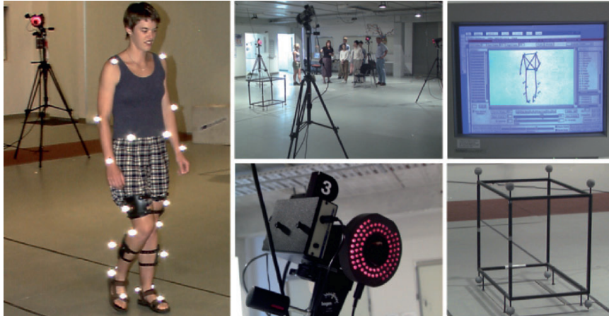
Fig. 1.13. Gait laboratory of The University of Auckland (in 2000). Left: walking subject with markers. Middle: walking area (top) and one of the fast cameras (bottom). Right: generated animated 3D stick figure (top) and camera calibration unit (bottom).
