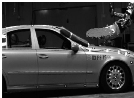
Fig. 19.12. Used tracks for multi-frame estimation in frame 200. All good tracks stay at the back area of the pedestrian that exhibits a rigid motion.
