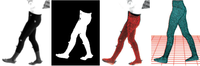
Fig. 13.9. From left to right: (a) Original image. (b) Silhouette. (c) Estimated pose. (d) 3D model.
