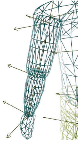
Fig. 14.2. One arm model with MPEG4 conformal joints as used in this work.
