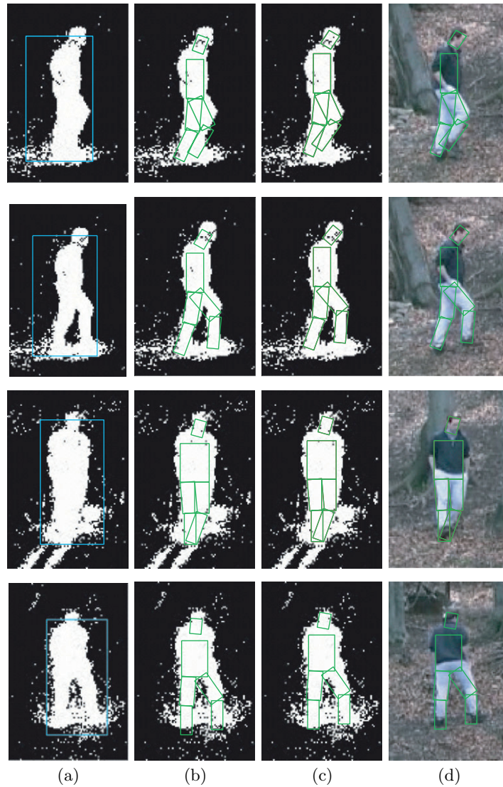
Fig. 5.8. ROI detection (a), model initialization (b), posture refinement (c) and outcome (d). Images of segmented motion are displayed as binary black and white images. Original data is displayed in the column (d). The found model is superimposed on both types of data. Courtesy A. Fexa for the sequence.
