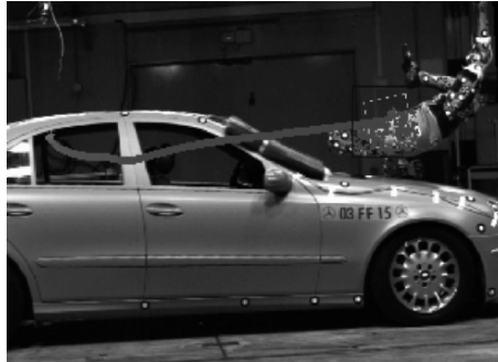
Fig. 19.13. KLT tracks on the same scene. Red (light) denotes large flow vectors, green (dark) small flows. the rotated rectangle shows the tracked region of interest.
