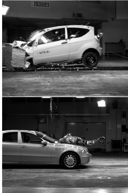
Fig. 19.4. Two typical crash test scenarios. EuroNCAP offset crash (left) and pedestrian crash (right).
